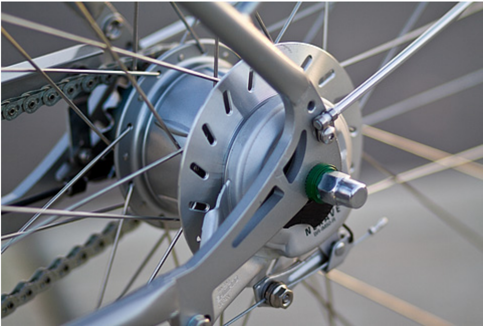
Figure 12 – Drum Brake system
