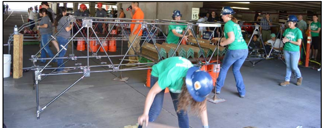
Figure 17: Vertical load test [3]
