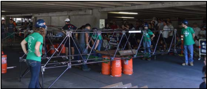
Figure 15: Lateral load test [3]
